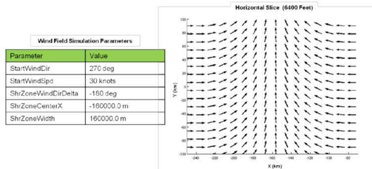
**Figure 9: Simulation Parameters and Generated Wind Field**
