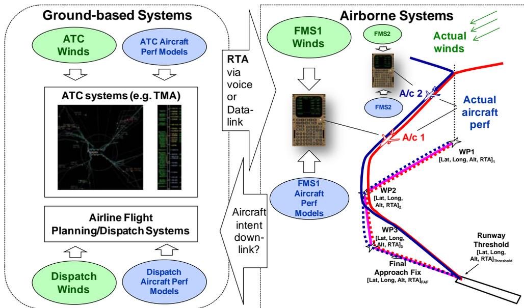
**Figure 3: Four Dimensional Trajectory-Based Operations Concept**
