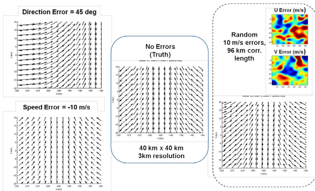
**Figure 10: Examples of Simulated Wind Forecast Errors**
