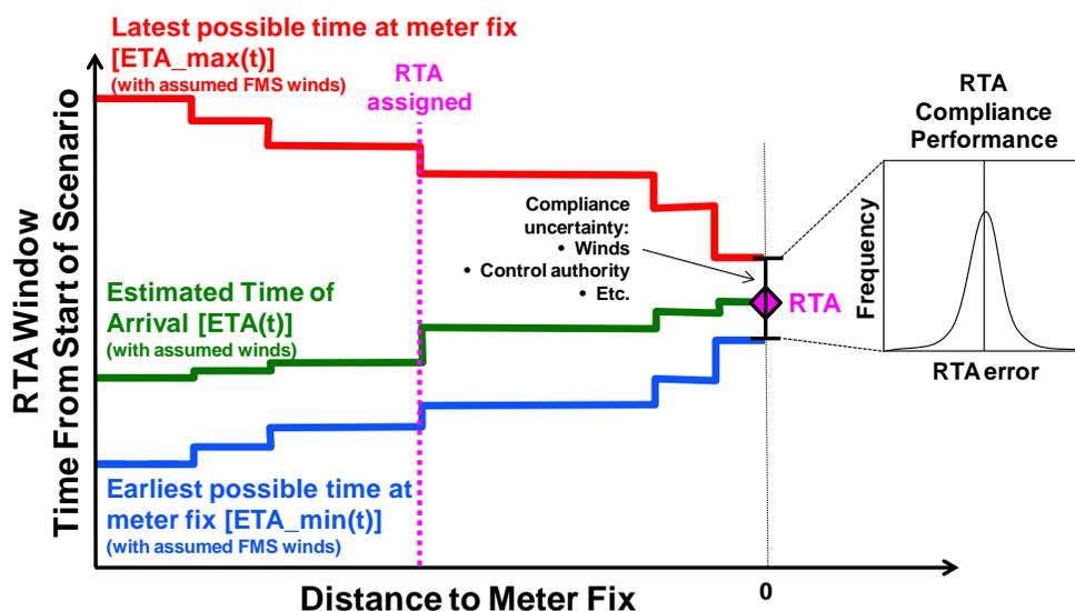
Figure 6: 4D-TBO RTA Window and RTA Compliance Performance Metrics
