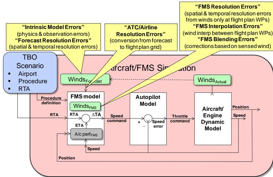
Figure 7: Key Wind Error Sources of Relevance to 4D-TBO Applications
