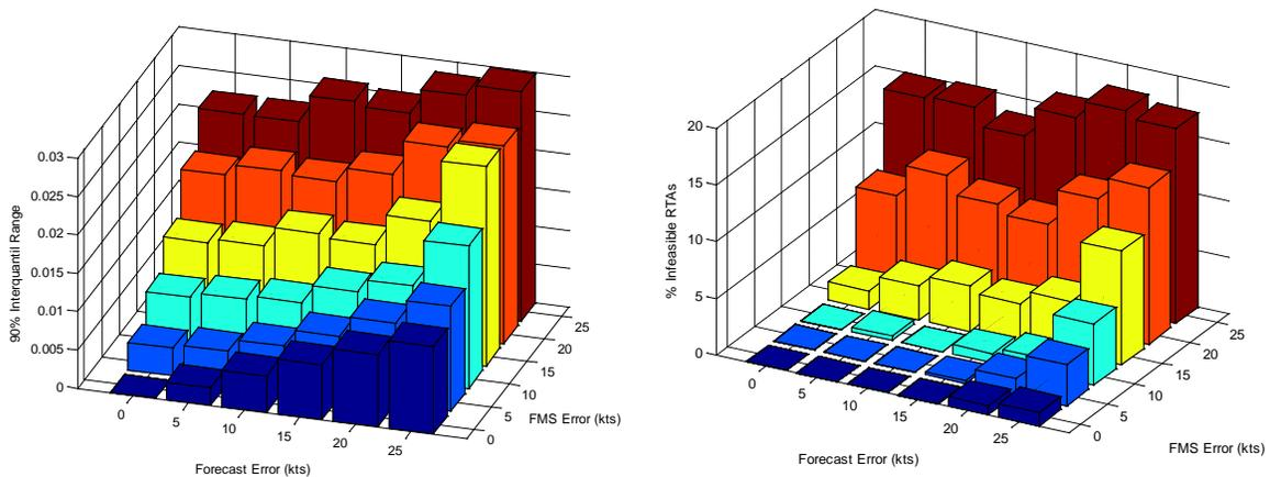
**Figure 13: RTA Compliance 90% Interquantile Range (left) and % Infeasible RTAs (right) as a Function of Forecast Wind Error and FMS Wind Error**
