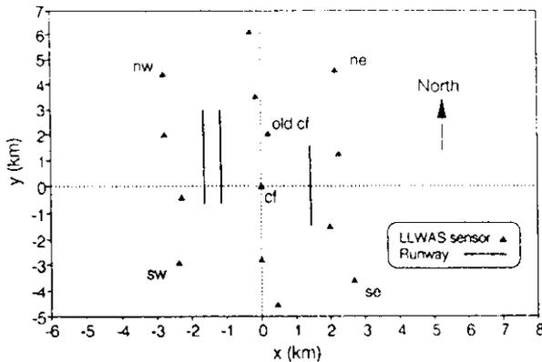
Figure 1. Schematic map of Orlando International Airport (MCO) showing runway and LLWAS sensor locations.
