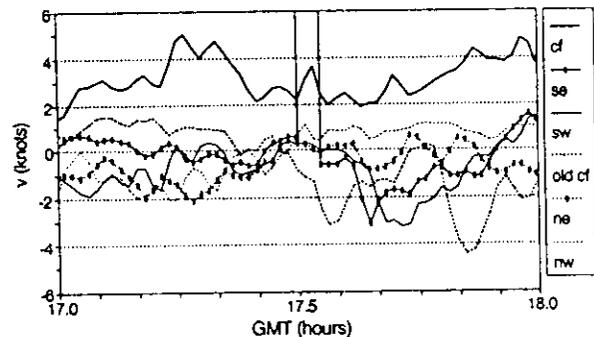
Figure 5. Measurements of the *v* wind component from 6 of the 14 MCO LLWAS sensors for a 1-hour period on 9/21/92, illustrating center field sensor bias. The vertical solid lines near 1730 GMT bound a data dropout in the southeast sensor.
