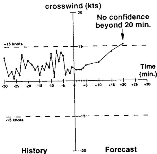
Figure 4. Tentative user display of crosswind series. In this example estimates of low forecast precision inhibit forecast displays for lead times greater than 20 minutes.
