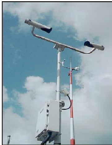
Figure 4: Example ASOS station configuration, the FD12P laser visibility sensor is shown at the top of the mounting pole.
