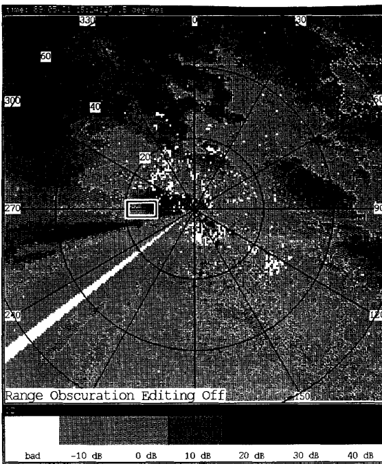
Fig. 6 TDWR Testbed Kansas City Reflectivity Data with Out-of-Trip Contamination. Microburst False Alarm is Indicated by Box.
