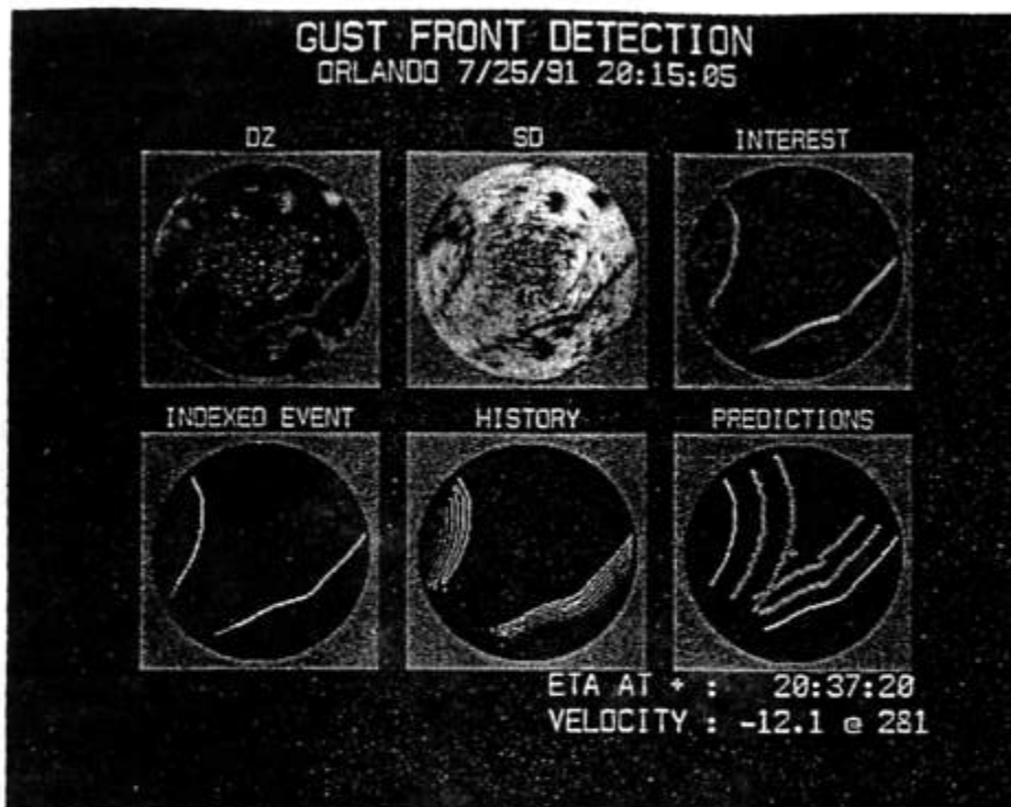
Figure 3. Summary of the results of processing a ASR-9 WSP scan containing two colliding gust fronts. (A) The reflectivity image DZ. (B) The image of local Doppler standard deviation SD. (C) The combined INTEREST image. (D) The set of extracted points called an EVENT. (E) The gust front points shown in the context of prior HISTORY. (F) The 10 and 20 minute PREDICTIONS of gust front location.
