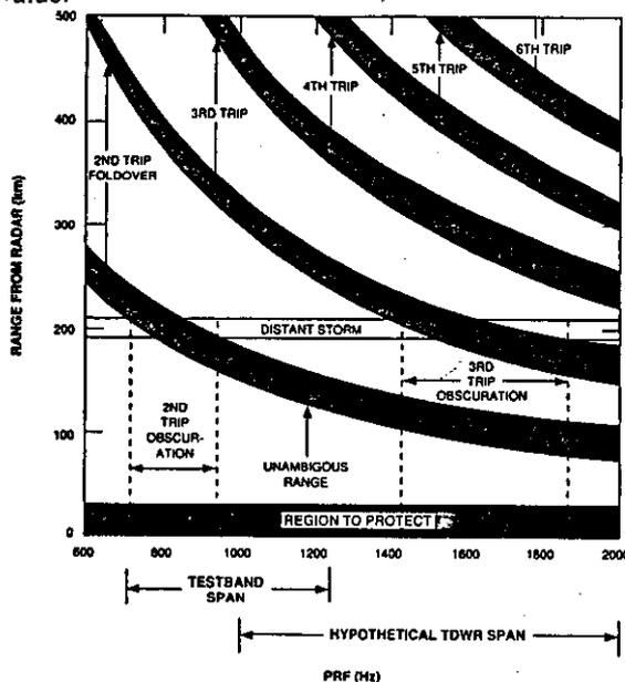
Figure 1. Adaptive PRF selection. The intersection of the lines containing the distant weather with the curves defining the nth trip foldover bounds indicate which PRF values will result in range contamination to the high priority region.
