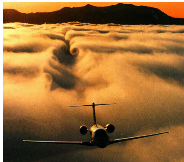
Figure 1: In this photograph, a Cessna Citation VI is flying immediately above a fog bank at approximately 313 km/h or 170 knots (B. Budzowski, Director of Flight Operations, Cessna Aircraft Company, private communication, 1993). Aircraft weight was approximately 8400 kg. As the trailing vortices descended over the fog layer due to the downwash, the flow field in the wake was made visible by the distortion of the fog layer. The aircraft is seen initiating a gentle climb after a level flight, leaving a portion of the fog layer yet unaffected. Photo courtesy of Cessna Aircraft Company. (Higuchi, 1993).
