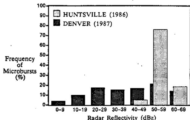
Fig. 1. Distribution of the maximum surface radar reflectivity factor in cells that produced microbursts.
