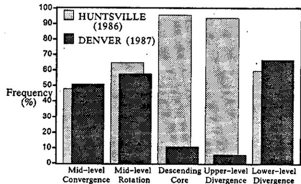
Fig. 6. Comparison of upper-altitude feature frequency for Huntsville and Denver microburst producing storms.
