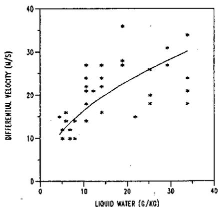
Fig. 2. Maximum radial velocity differential plotted against liquid water content for Huntsville.
