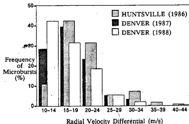
Fig. 3. Distribution of the maximum radial velocity differential across microbursts observed in real time.
