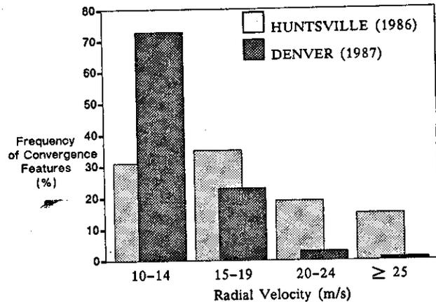
Fig. 8. Frequency of mid-level convergence as a function of radial velocity.
