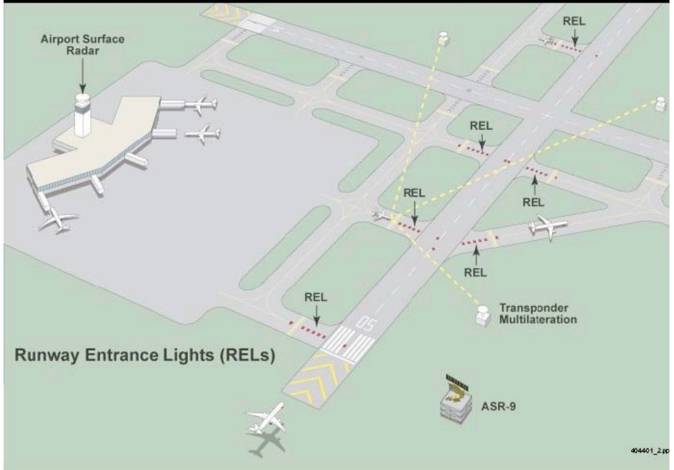
Figure 2 Conceptual diagram of the Runway-Status Light System at DFW and SAN with surveillance sources driving red RELs. (note SAN does not have multilateration)
