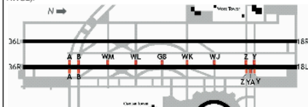
Figure 2 DFW west side with REL alignment and locations on 18L/36R taxiway intersections.
