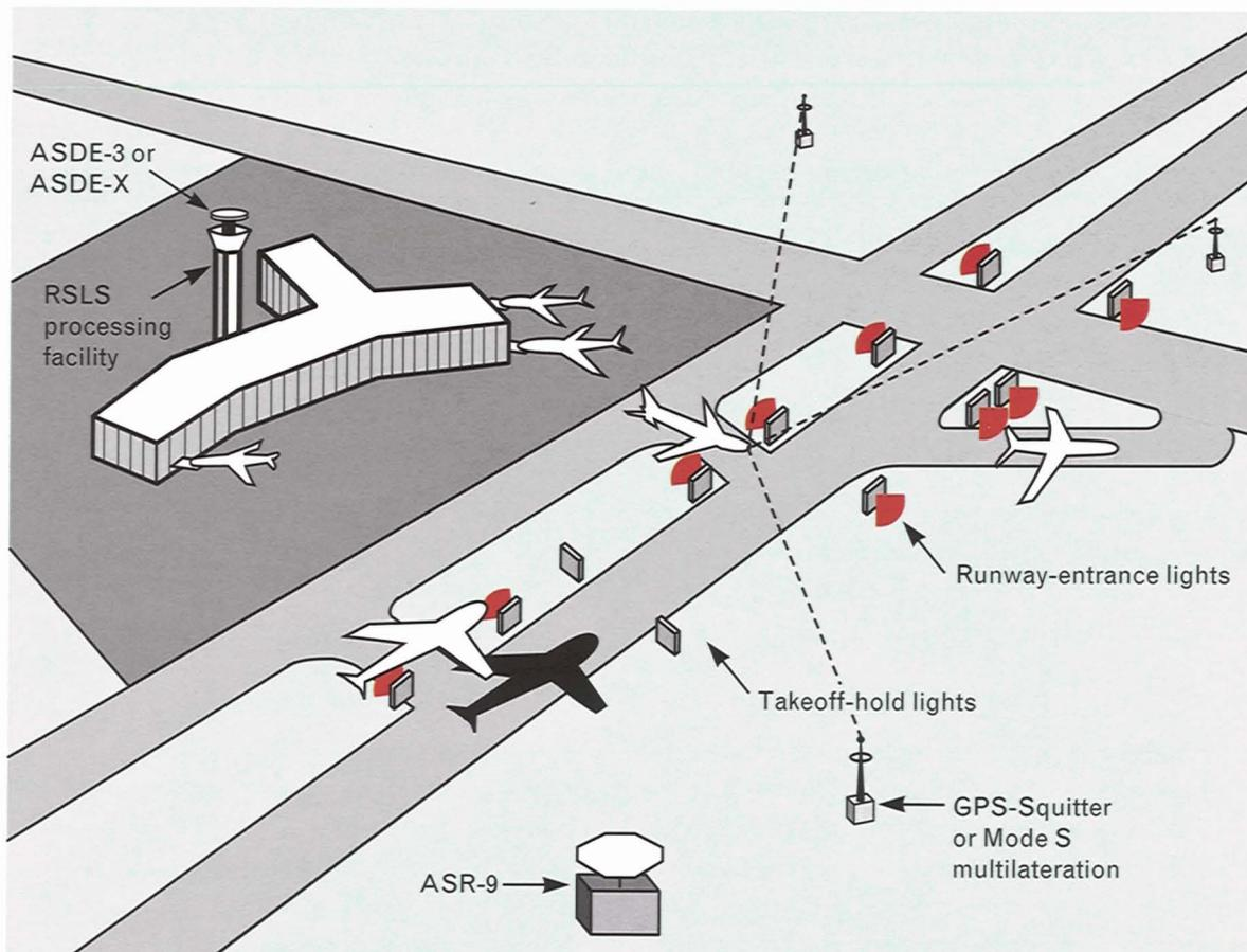
**FIGURE 1.** Runway-status light system (RSLs) concept. The runway-status lights indicate to aircraft pilots and surface-vehicle operators when the runway is unsafe to enter or unsafe for takeoff. The system is operated automatically, based on surveillance provided by an Airport Surface Detection Equipment (ASDE) surface radar, an Airport Surveillance Radar (ASR-9) approach radar, and future surveillance systems such as GPS-Squitter or Mode S multilateration.
