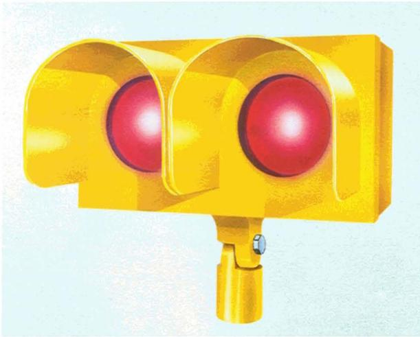
**FIGURE 2.** A proposed runway-status light fixture. This fixture is based on the standard International Civil Aviation Organization taxi hold-position (wig-wag) light, with the amber lenses replaced by red lenses and the lamps upgraded to brighter bulbs. An addressable light controller would be mounted in or near the base of this fixture to allow individual control over each lamp.
