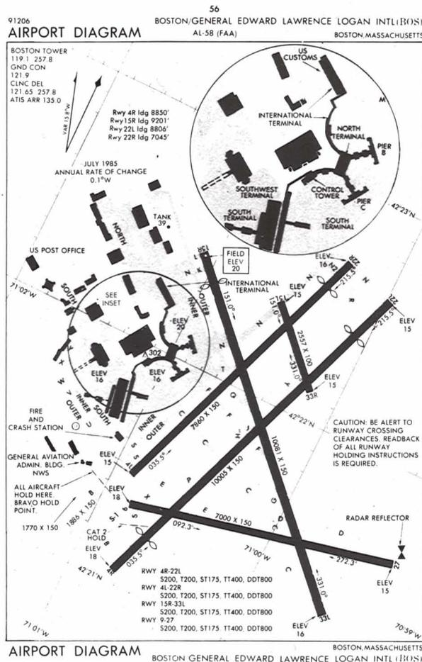
**FIGURE 7.** Boston Logan International Airport runway and taxiway map. The runways and buildings are shown in black and the taxiways are shown in gray. The taxiway configuration is shown as of 1992; some new taxiway construction and change in nomenclature has occurred since this map was produced.
