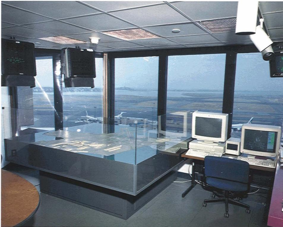
**FIGURE 8.** RSLS Logan Demonstration room. The windows offer a sixteenth-floor view of Logan Airport and Boston harbor. The RSLS model board is on the left, while the computer monitors are on the right. The two displays above the model board are high-brightness monochrome displays used to show the traffic in and near the airport.
