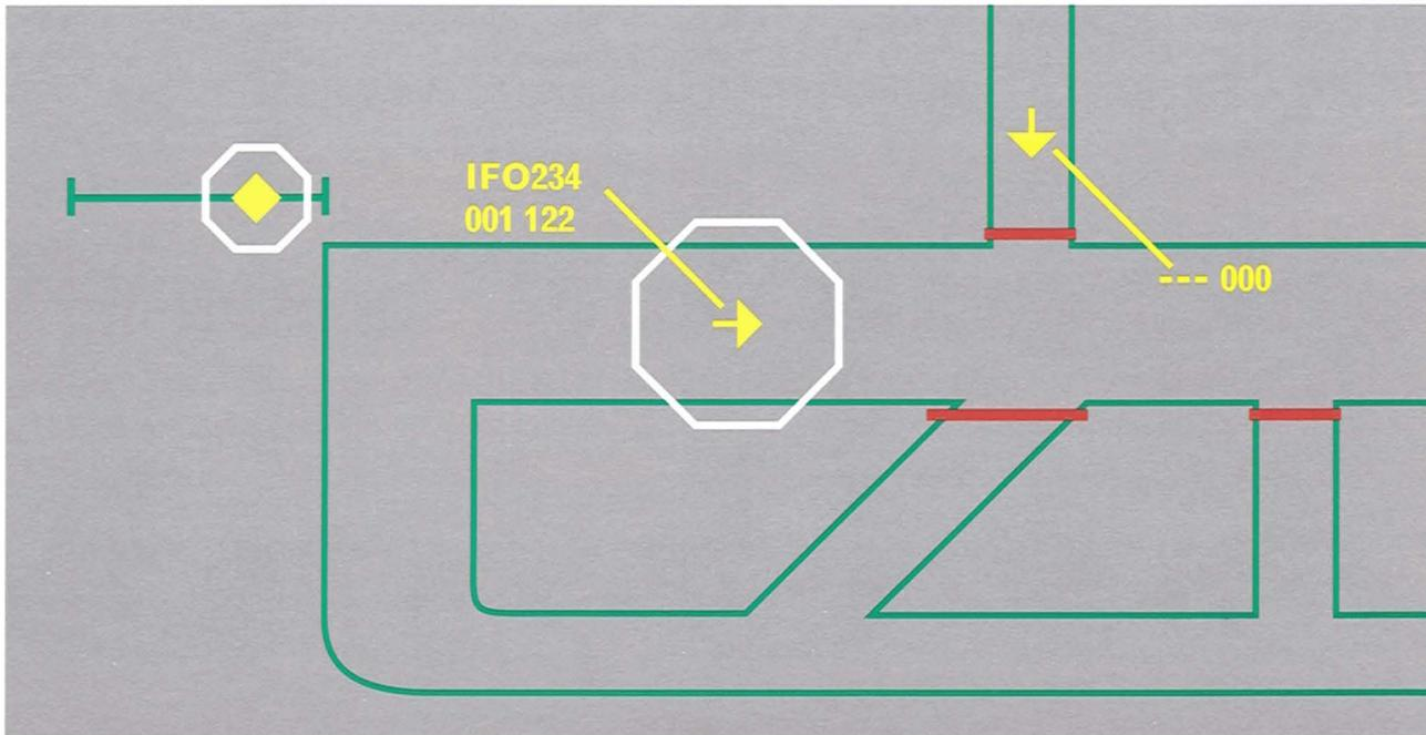
**FIGURE 5.** RSLs enhancements to the ASDE controller display. Arrows indicate position, direction of motion, and size of the radar tracks. Stationary tracks are also optionally depicted by circles. Data tags present the radar track's altitude, velocity, flight number, and equipment type. The approach bar depicts an aircraft on approach to a particular runway; its two endpoints represent approximately five miles of airspace from the outer marker to the runway threshold.
