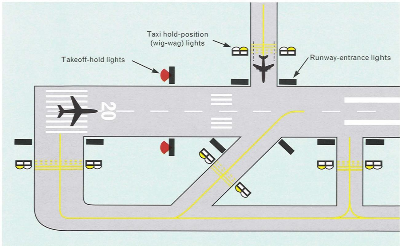
**FIGURE 4.** Takeoff-hold lights in operation for an aircraft in position for departure with crossing traffic. The takeoff-hold lights indicate that the runway is currently unsafe for departure because the runway is about to be occupied by a crossing aircraft.
