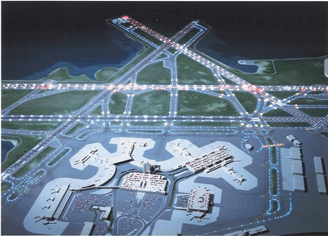
**FIGURE 9.** RLSL Logan Demonstration model board. The model board is an architectural model of Logan Airport with computer-controlled fiber optic lights simulating the runway-status lights; runway approach, threshold, centerline, and edge lights; taxiway centerline and edge lights; and taxi hold-position lights. All of the runway lights are illuminated in this photograph, which is for illustration only and does not represent any real runway configuration.
