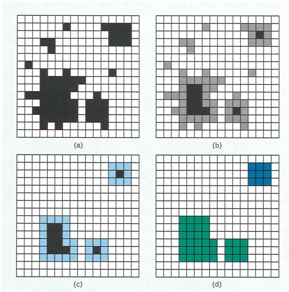
**FIGURE 10.** Morphological processing example. (a) In the input radar image, the black squares denote clutter-rejected target pixels. (b) Erosion deletes the pixels marked in gray. (c) Subsequent dilation adds the pixels marked in light blue. (d) The two green components are close enough to be grouped as a single object. The blue component is a separate object.
