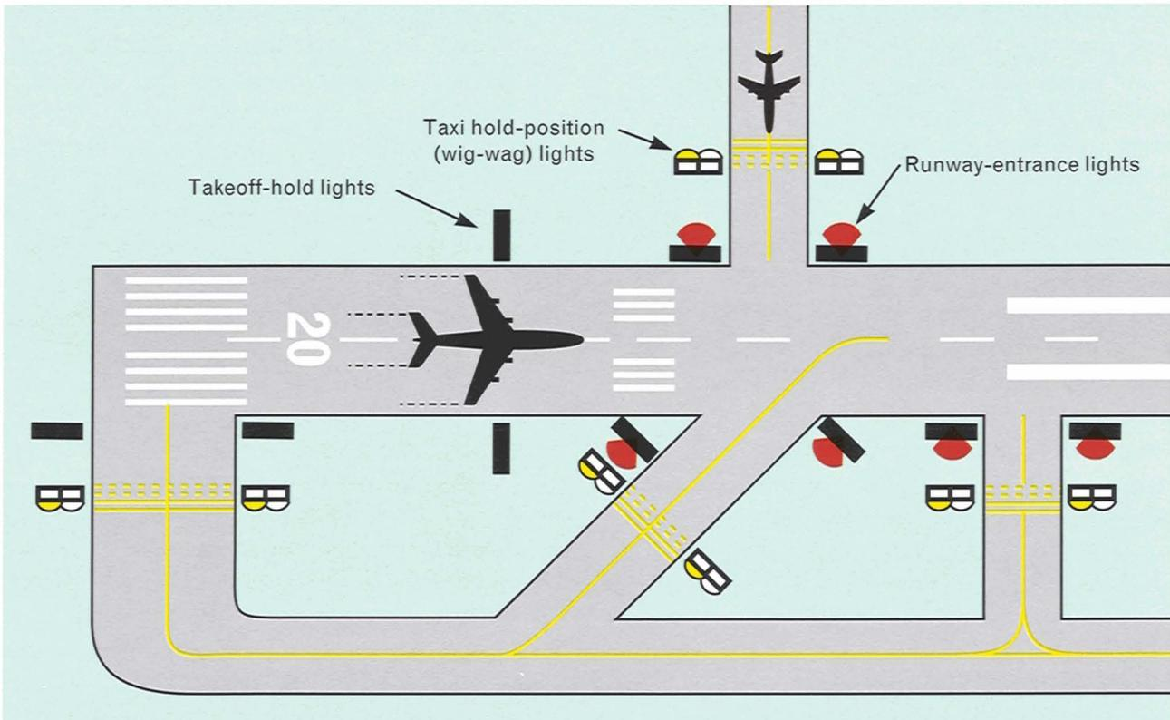
**FIGURE 3.** Runway-entrance lights in operation for an aircraft landing on a runway. The runway-entrance lights in front of the landing aircraft are illuminated red, indicating to the taxiing aircraft that the runway is unsafe to enter. The runway-entrance lights behind the landing aircraft are extinguished, indicating that the runway is safe to enter there.
