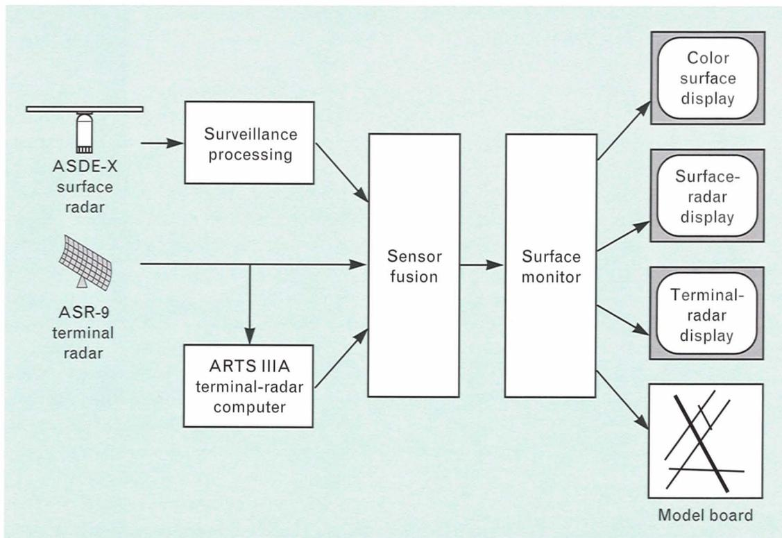
**FIGURE 6.** Overview of the RSLS Logan Demonstration architecture. Surveillance provided by a surface radar and a terminal radar is processed separately and then fused to provide aircraft tracks on the airport surface and in the approach space. The surface monitor assesses the traffic picture and drives the runway-status lights. The different displays show the traffic and runway-status light information on a map of the airport and its vicinity.
