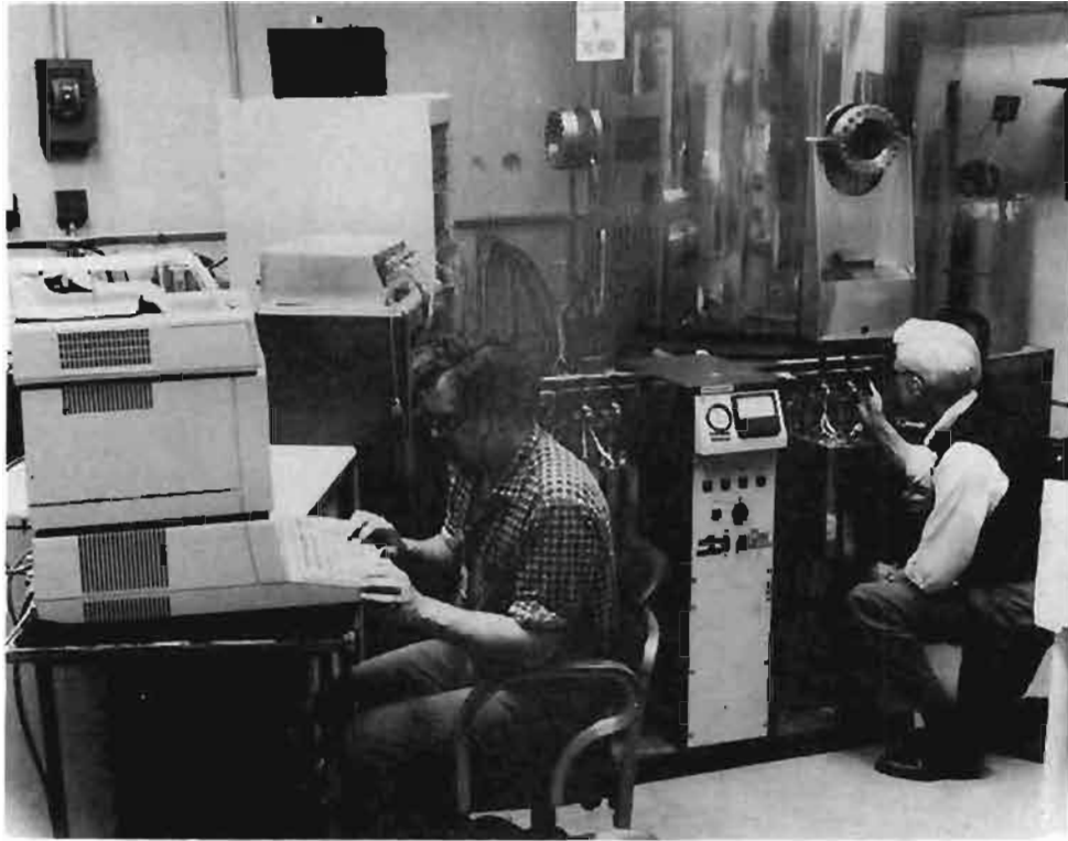
Figure III-13. View of Ultek pressure (vacuum) chamber at M.I.T. Lincoln Laboratory. Chamber is sealed and in operation. Operator at keyboard is using the HP Automatic Data Acquisition System.
