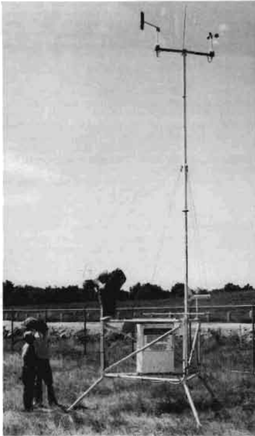
Figure II-7. View of automatic weather station features not shown in Figure II-6. Technician is working on antenna. Notice wind sensor mast is self-guyed.
