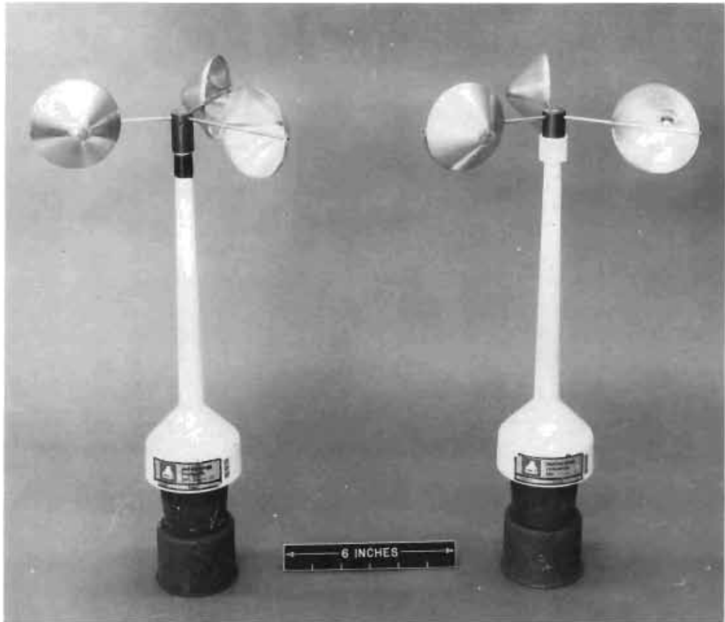
Figure III-2. Anemometer hubs, to which cups are attached, are shown both before (left) and after (right) modification. Notice at right how the white Teflon bushing extends down from the black hub and covers the O-ring (shown in Figure III-1).
