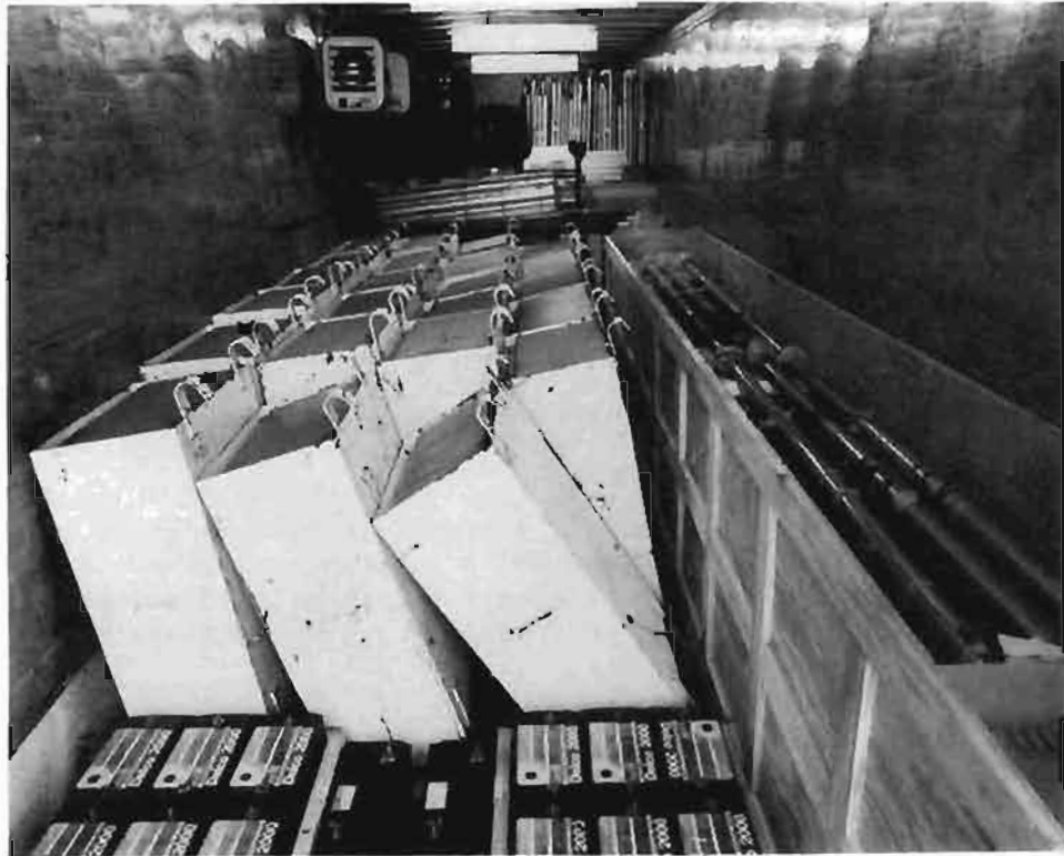
Figure A-2. View looking into the truck trailer used to transport FLOWS mesonet equipment. Fluorescent lighting and a heater (upper left) have been added. Note the long wind sensor masts (right), the white armored boxes (left), and the batteries (front).
