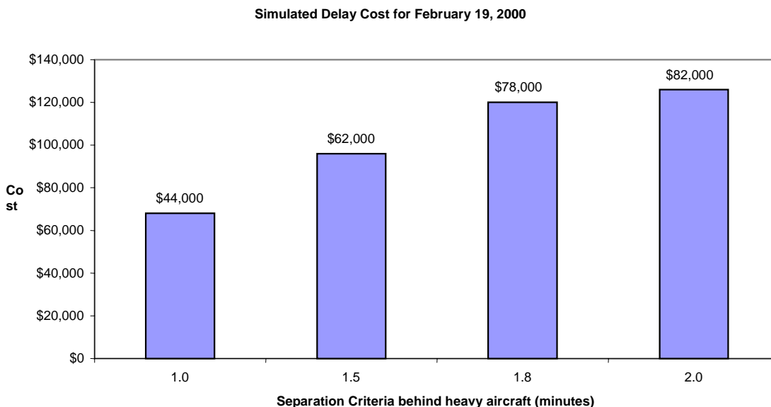
Figure 8. Simulated delay cost at DFW for different separation criteria on February 19, 2000.
