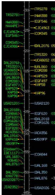
Figure 2-2. TMA TGUI display, showing the ETA (left) and STA (right, with assigned delay) for each flight metered to the Boston Logan airport arrival runway between 45 minutes after the current hour until 30 minutes after the following hour. Flights with blue STAs are inside the Freeze Horizon while yellow STAs depict flights still beyond the Freeze Horizon.
