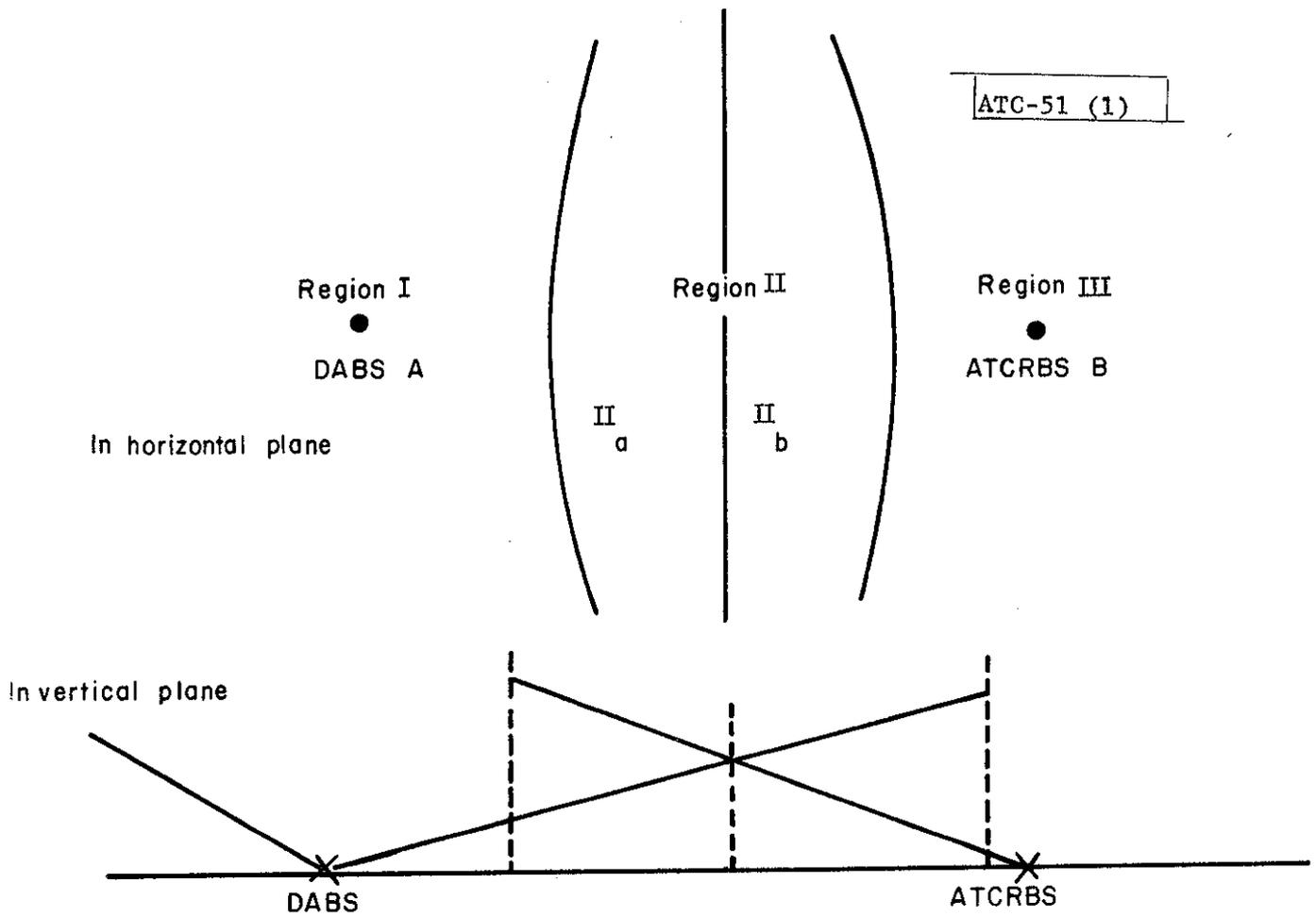
Fig. 1 Coverage in a DABS boundary zone.
