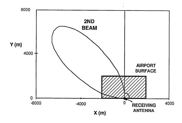
Figure C-2. Interference region within second beam.
