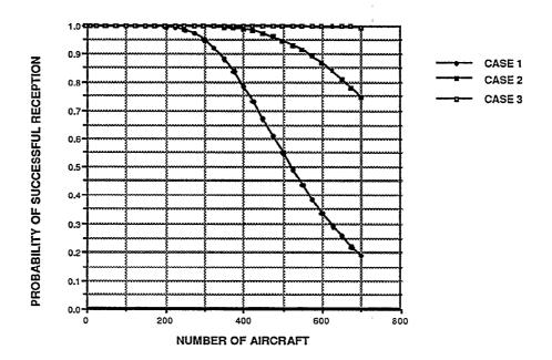
Figure 2-5. 6-sector detection probability over 5 seconds.
