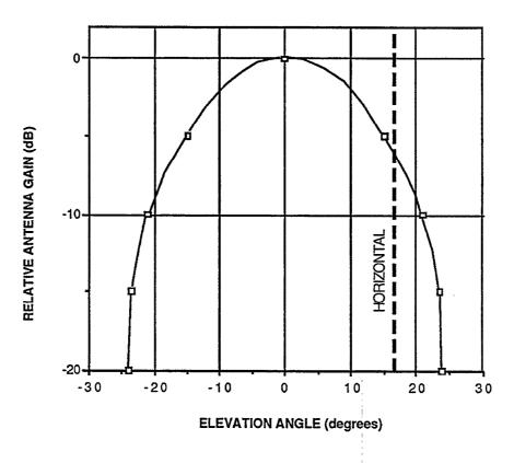
Figure B-2. Vertical antenna patterns.
