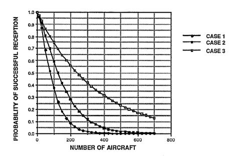
Figure 2-1. Omni detection probability each half second.
