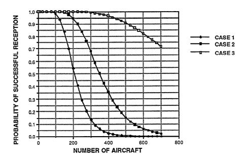
Figure 2-3. Omni detection probability over 5 seconds.
