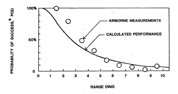
\* PERCENT OF AIRCRAFT FROM WHICH REPLIES ARE ELICITED BY A 4-WATT INTERROGATION, FOR AIRCRAFT WITHIN ± 10° IN ELEVATION ANGLE
