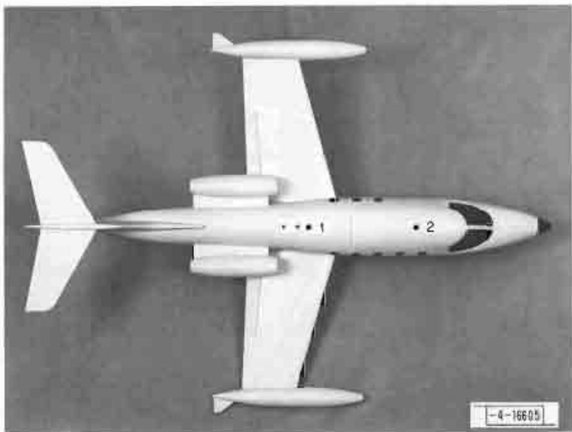
Fig. I-18. Gates Lear Jet, top view showing antenna positions 1 and 2.
