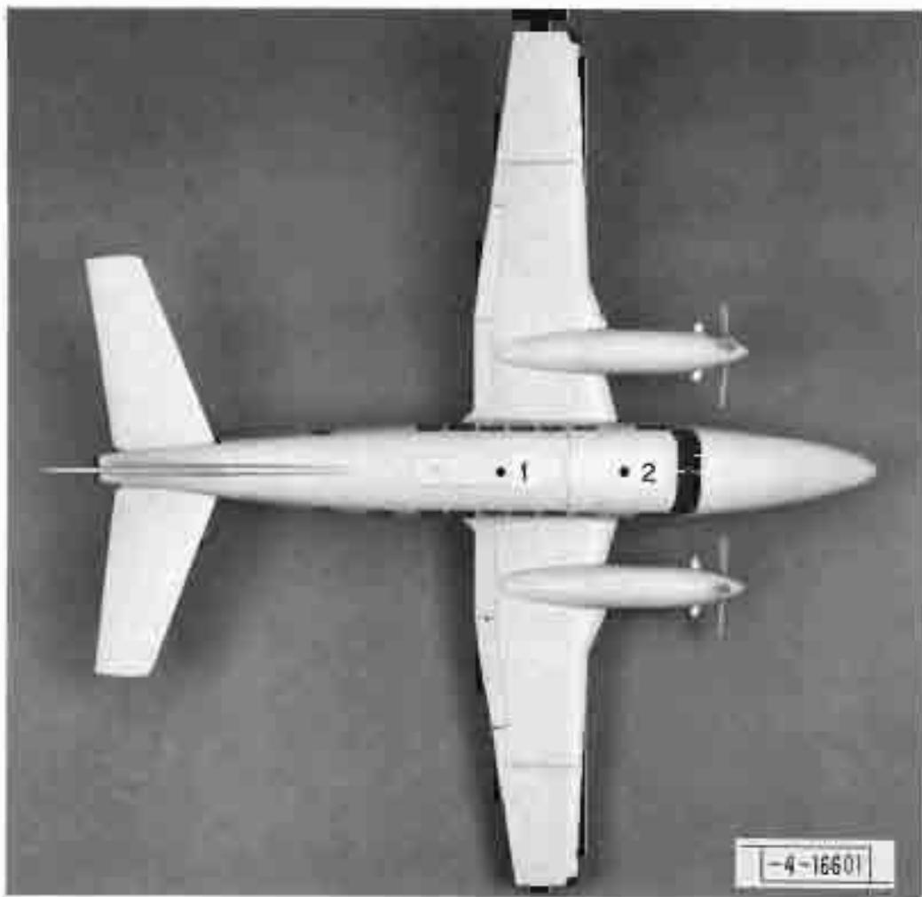
Fig. 1-15. Beechcraft B99, top view showing antenna positions 1 and 2.
