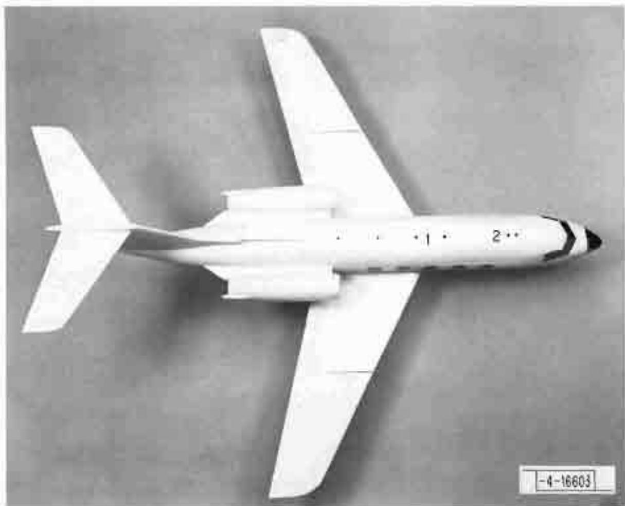
Fig. 1-21. Grumman Gulfstream, top view showing antenna positions 1 and 2.
