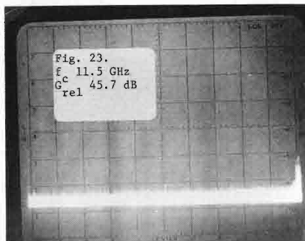
Figs. 21-24. Coaxial magnetron (QKH-1739LL) operated at 2.7 GHz (V-axis: 10 dB/div; H-axis: 100 MHz/div).
