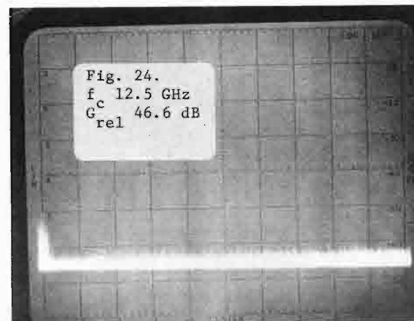
Figs. 21-24. Coaxial magnetron (QKH-1739LL) operated at 2.7 GHz (V-axis: 10 dB/div; H-axis: 100 MHz/div).
