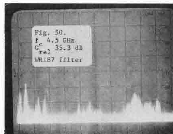
Figs. 47-50. Coaxial magnetron (QKH-1739LL) operated at 2.9 GHz (V-axis: 10 dB/div; H-axis: 100 MHz/div).
