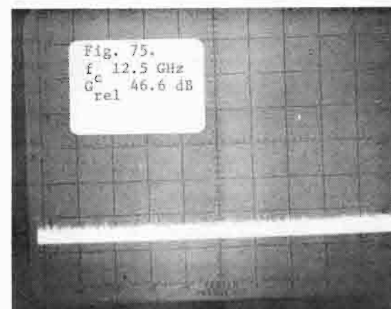
Figs. 72-75. Conventional magnetron (DX-276) operated at 2.7 GHz (V-axis: 10 dB/div; H-axis: 100 MHz/div).
