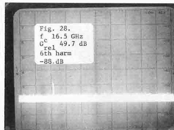
Figs. 25-28. Coaxial magnetron (QKH-1739LL) operated at 2.7 GHz (V-axis: 10 dB/div; H-axis: 100 MHz/div).
