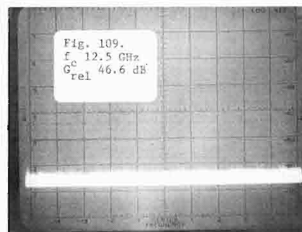
Figs. 106-109. Conventional magnetron (DX-276) operated at 2.9 GHz (V-axis: 10 dB/div; H-axis: 100 MHz/div).
