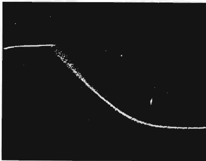
Fig. 119. Front edge of RF envelope - no priming (V-axis: linear power - not calibrated; H-axis: 50 nsec/div).
