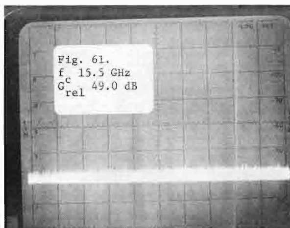
Figs. 59-62. Coaxial magnetron (QKH-1739LL) operated at 2.9 GHz (V-axis: 10 dB/div; H-axis: 100 MHz/div).
