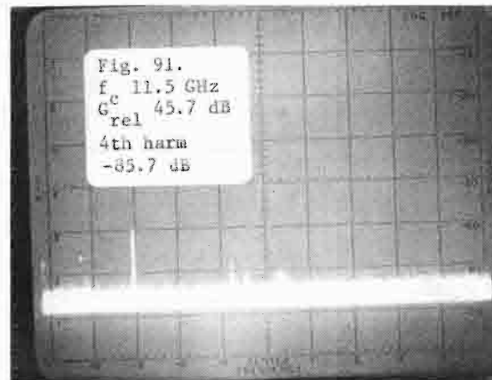
Figs. 89-92. Conventional magnetron (DX-276) operated at 2.8 GHz (V-axis: 10 dB/div; H-axis: 100 MHz/div).
