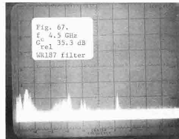
Figs. 64-67. Conventional magnetron (DX-276) operated at 2.7 GHz (V-axis: 10 dB/div; H-axis: 100 MHz/div).
