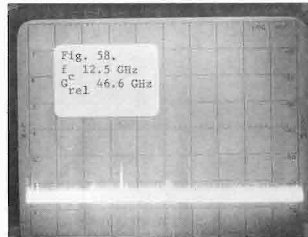
Figs. 55-58. Coaxial magnetron (QKH-1739LL) operated at 2.9 GHz (V-axis: 10 dB/div; H-axis: 100 MHz/div).
