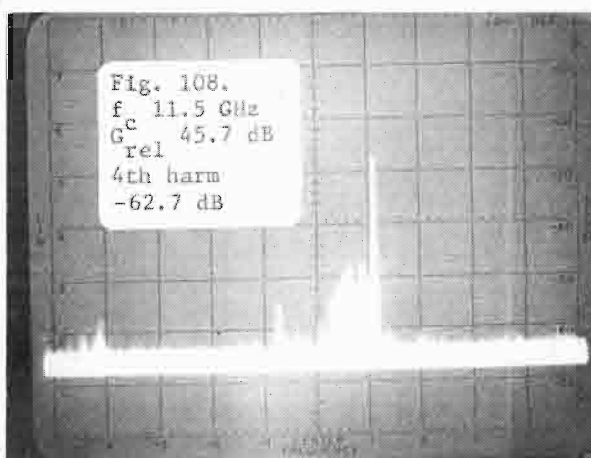
Figs. 106-109. Conventional magnetron (DX-276) operated at 2.9 GHz (V-axis: 10 dB/div; H-axis: 100 MHz/div).
