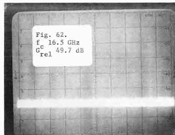
Figs. 59-62. Coaxial magnetron (QKH-1739LL) operated at 2.9 GHz (V-axis: 10 dB/div; H-axis: 100 MHz/div).
