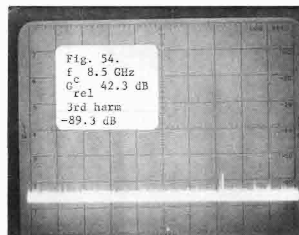
Figs. 51-54. Coaxial magnetron (QKH-1739LL) operated at 2.9 GHz (V-axis: 10 dB/div; H-axis: 100 MHz/div).
