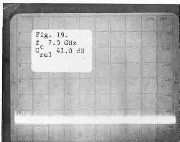
Figs. 17-20. Coaxial magnetron (QKH-1739LL) operated at 2.7 GHz (V-axis: 10 dB/div; H-axis: 100 MHz/div).
