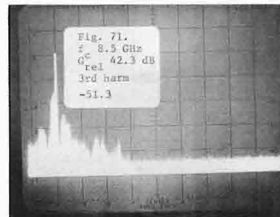
Figs. 68-71. Conventional magnetron (DX-276) operated at 2.7 GHz (V-axis: 10 dB/div; H-axis: 100 MHz/div).
