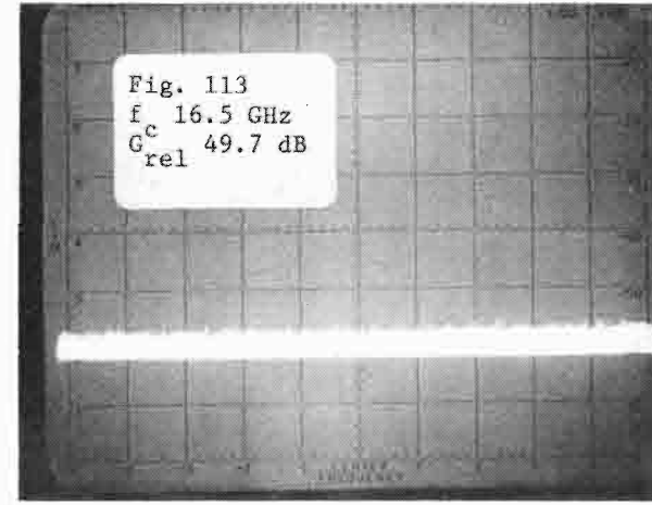
Figs. 110-113. Conventional magnetron (DX-276) operated at 2.9 GHz (V-axis: 10 dB/div; H-axis: 100 MHz/div).
