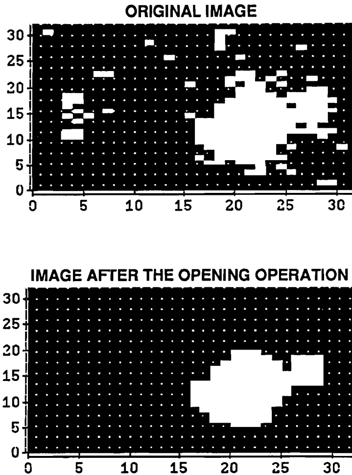
Figure 3-3. The effect of the morphological opening process on an image.
