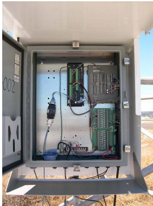
Figure 5. Data logger system housed inside equipment box.
