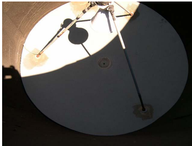
Figure 4. Sodar antenna viewed looking down into baffle.
