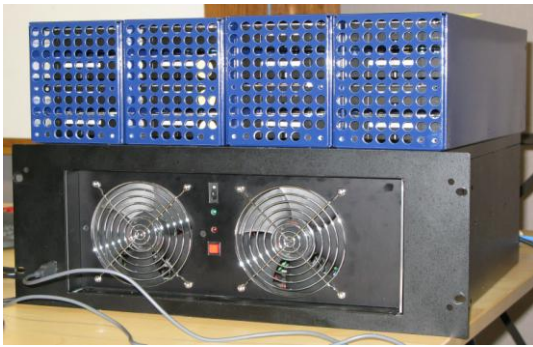
Fig 2 Streaming data system with 96TByte (4x24Tbyte) disk-packs capable of 4.4Gbyte/s continuous record (8Gbyte/s bursts) or playback.
