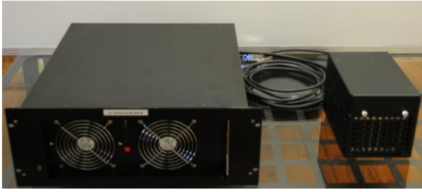
Fig 1 Streaming data system (19" 4U 17"D) together with a 16 TByte disc pack. Several form factors and level of ruggedness are available (half rack, helicopter version).
