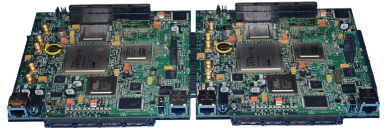
2 Processor modules connected side-by-side, each with a PowerPC and Virtex-6.
