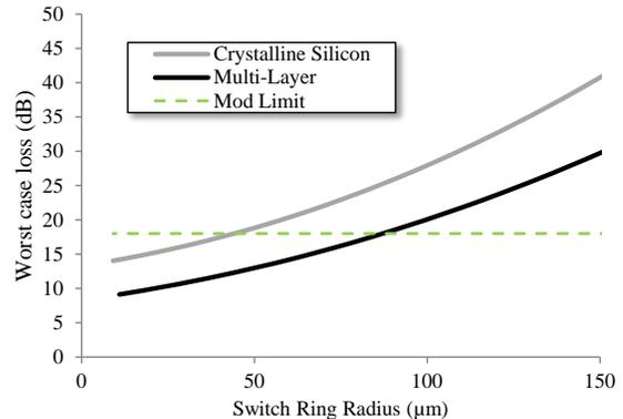
Fig. 3. Comparison of insertion loss between crystalline silicon and multi-layer implementations.
