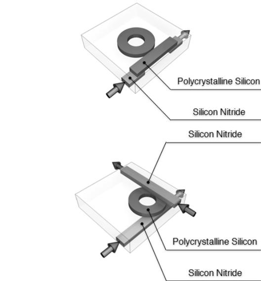
Fig. 1. Arrangement of silicon nitride and polysilicon for making multi-layer ring resonators.
