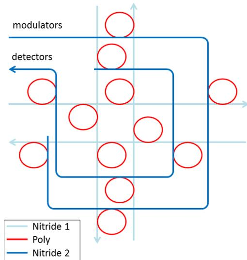
Fig. 2. Layout of photonic switch tile, showing waveguides and ring resonators.
