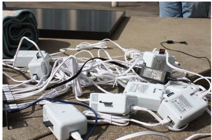
Figure 4: Pile of 10 SheevaPlugs powered by a solar panel in the background. Even with a power-hungry switch this ran at well under 100W.
