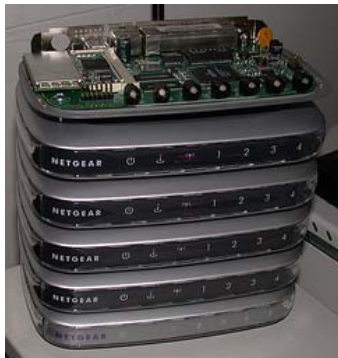
Figure 1: “Microclusters” of the WGT634u. One of our test setups created a tree of 35 nodes; seven sub-clusters of five nodes each. This was so we could fully involve an 8 port switch (counting uplink to the head node).
