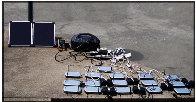
Figure 3: 16 of the WGT634u intercommunicating via 802.11g and 802.11s. This was with the primary bandwidth test device, wlan0, which becomes mesh0 under 802.11s.
