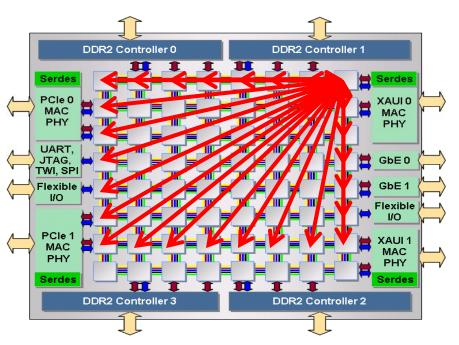
iLib messages were sent from a single tile to a "ring" of receiver tiles using the available channels (raw, streaming, buffered) for a varying number of packets and payload sizes.
