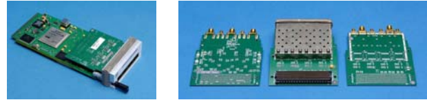
Figure 2: A radar frontend FPGA processor and its FMC boards.
