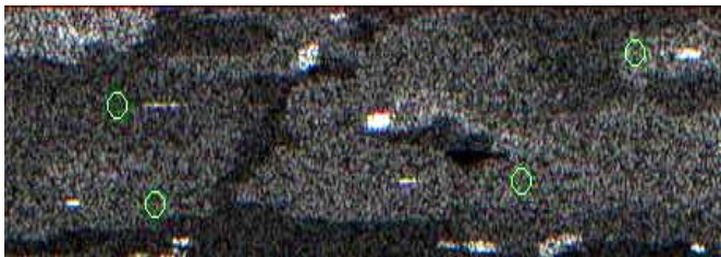
Figure 1: Part of a typical SAR image showing shifting and blurring of four moving targets.
