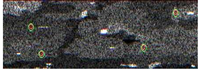
Figure 2: SARMTI has correctly determined the actual positions of the moving targets (red circles) from the same SAR image data
