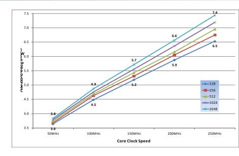
1D FFT performance up to 20 GFLOPS, 2D FFT performance up to 16 GFLOPS 1D convolution performance up to 22 GFLOPS, ~3 GFLOPS/watt on FFTs
