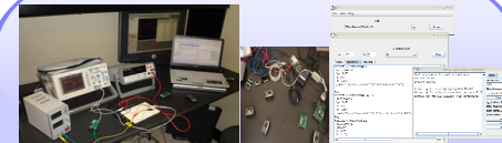
Figure 1 Setup for the power measurement; the USB attached mote acts as the Cluster Head, the other motes are distributed around the laboratory. A Java GUI was built to provide user friendly environment to deal with the motes.
