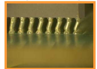
After 1500 Thermal Cycles
