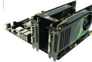
Figure 1: Example dual GPU solution.
