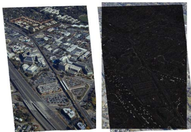
Figure 2: Affine warp versus dense correspondence. Top: source and target images. Middle: affine warp with difference image. Bottom: dense correspondence warp with difference image (significant differences are movers).
