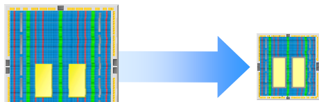
Figure 2: HardCopy Die Change (Stratix III FPGA to HardCopy Device)
