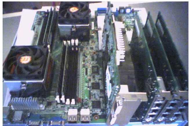
Figure 1: A measure polytope node has some number of NICs appropriate to the cluster scale with the first NIC being used for the most latency sensitive traffic.
