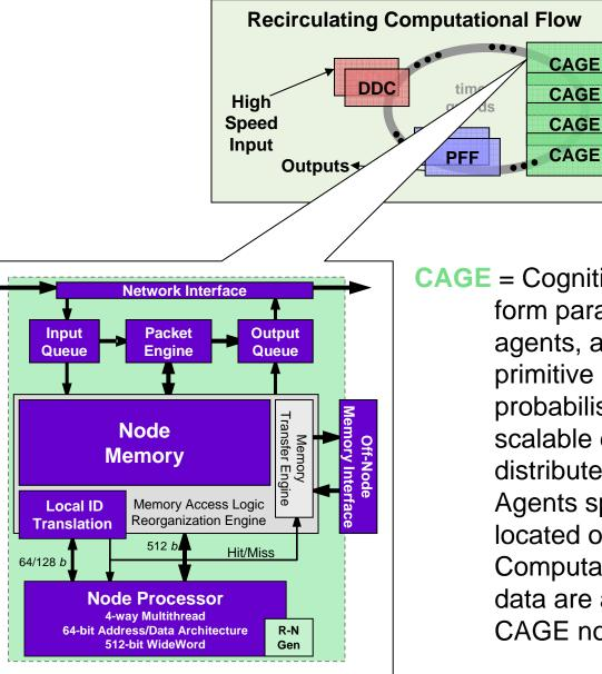
CAGE = Cognitive Agent & Graph Engine(s) – form parallel computing fabric, hosts agents, augmented ISA accelerates primitive operations on graphs, supports probabilistic reasoning, uses distributed, scalable data storage; Agents distributed to 1 or more CAGE nodes, Agents spawn cognitive functions located on 1 or more CAGE nodes, Computations requests on non-local data are automatically sent to proper CAGE node via PFF & DDC
