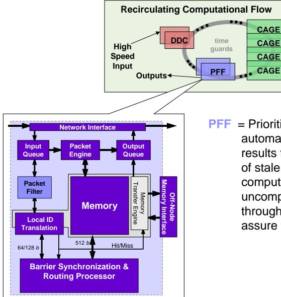
PFF = Prioritize, Filter and Fuse – automatic "gather"/ coalescing results from CAGE(s), pruning of stale and unproductive computation, re-circulates uncompleted computations through DDC, time based to assure timely results
