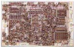
Intel 4004, 10 microns 2300 transistors (1971)
