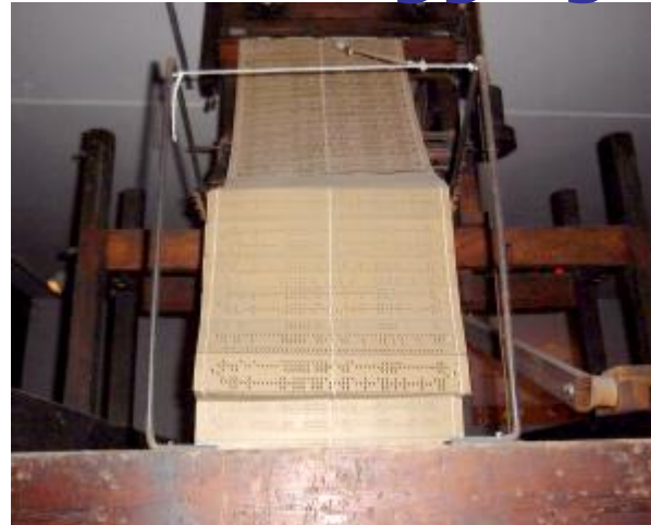
Punch Cards (textile loom 1840)
