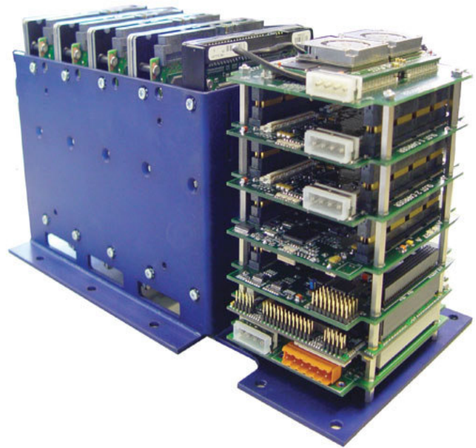
Figure 11 – HPEC application using Nallatech FPGA COTS products [9]
