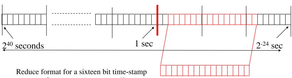
horizon 2<sup>-2</sup> seconds, granularity 2<sup>-18</sup> seconds
