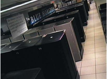
On February 9, 2000 IBM formally dedicated <u>Blue Horizon</u>, the teraflops computer. <u>Blue Horizon</u> has 42 towers holding 1,152 compute processors, and occupying about 1,500 square feet. Blue Horizon entered full production on April 1, 2000.
