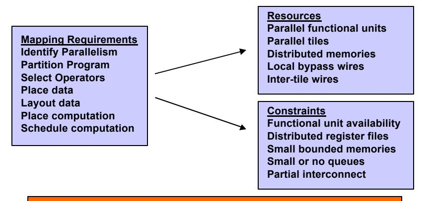
Increasing the arithmetic/memory ratio while holding silicon area fixed simultaneously increases resources and tightens constraints.
