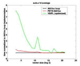
The horizontal axis is  $log_2 N$ . The vertical axis is the time required by each implementation to perform the operation, normalized to the time of the hand coded AltiVec loop implementation, averaged over many iterations.
